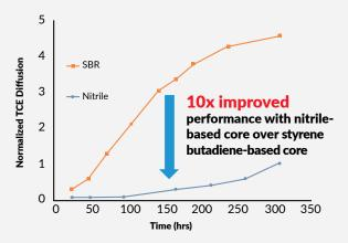
Accelerated comparison of the TCE vapor resistance of Nitra-Core, a nitrile-modified spray applied asphalt layer, against spray-applied asphalt latex core, a styrene butadiene-modified asphalt layer. Both asphalt layers were sprayed to an identical thickness for the test.
