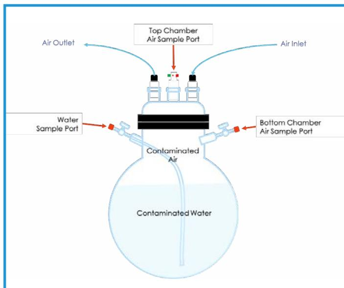
**Figure 1.** Vapor-Barrier Testing Apparatus
