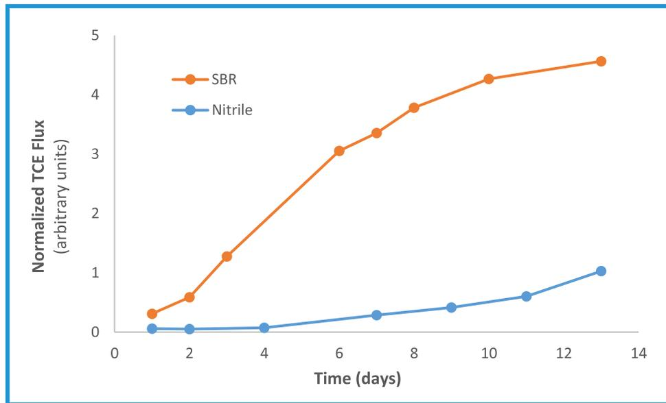
**Figure 2.** Accelerated comparison showing relative TCE flux compared to the two polymer-modified spray-applied asphalt layers tested over time. SBR = styrene butadiene modified-asphalt, nitrile = acrylonitrile butadiene-modified asphalt. Both asphalt layers were sprayed to an identical thickness (20 mil) for the test.
